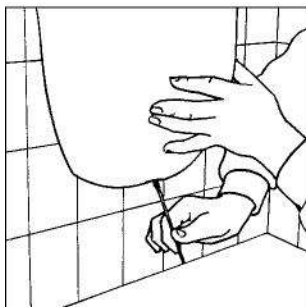
9 Install the trap cover against the lavatory and draw the screw tap downwards.
